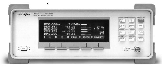
The Agilent 86120C Multi-Wavelength Meter is a Michelson interferometer-based instrument that measures wavelength and optical power of laser light in the 1270 to 1650 nm wavelength range. Simultaneous measurements of multiple laser lines are performed allowing measurements of DWDM signals and multiple lines of Fabry-Perot lasers. Each laser line is assumed to have a linewidth (including modulation sidebands) of less than 5 GHz.
